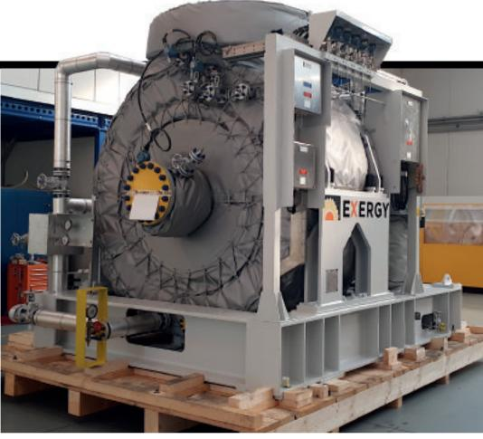
The lube and seal oil console by Exergy is compliant with API technical standards for oil & gas applications.
